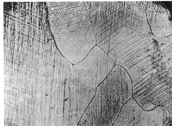
Figure 3.10. Rosenhain's micrograph showing slip lines in lead grains.
